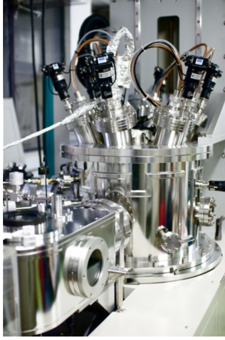
Figure 3.1: Picture of the magnetron sputtering system.
